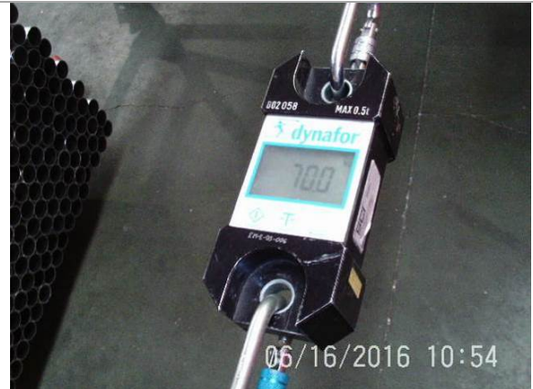
42. Measure of horizontal load at midrail (70Kg / 154.35lbs)
