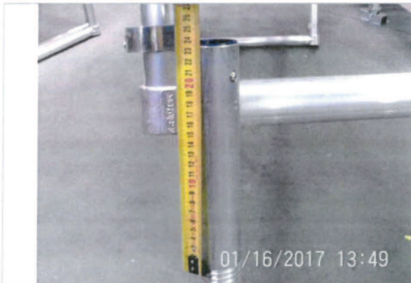
49. Screwjacks measure (inside part)
