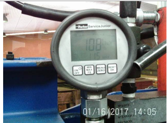
48. Caster load test (16.95kN)
