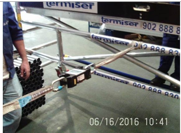
40. Horizontal load at handrail
