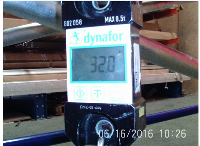
36. Measure of vertical load (32Kg / 70.56lbs)
