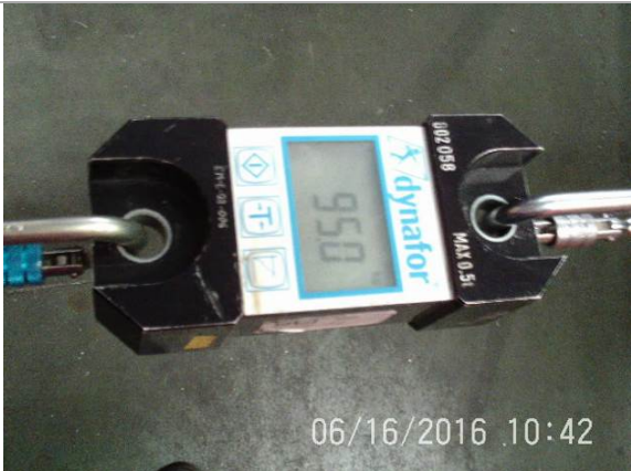
41. Measure of horizontal load at toprail (95Kg / 209.47lbs)
