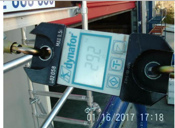
34. Measure of horizontal load (29.2Kg / 64.37lbs)
